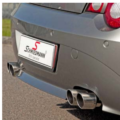
Right: Full exhaust systems are available for the Z4, from the manifold to high-flow cats and stainless steel cat-back systems.
