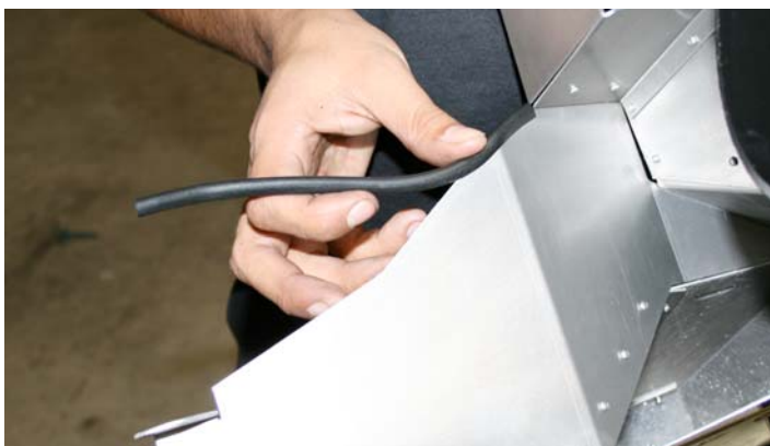
12- Install the supplied trim seal to the lower edge of the housing.
