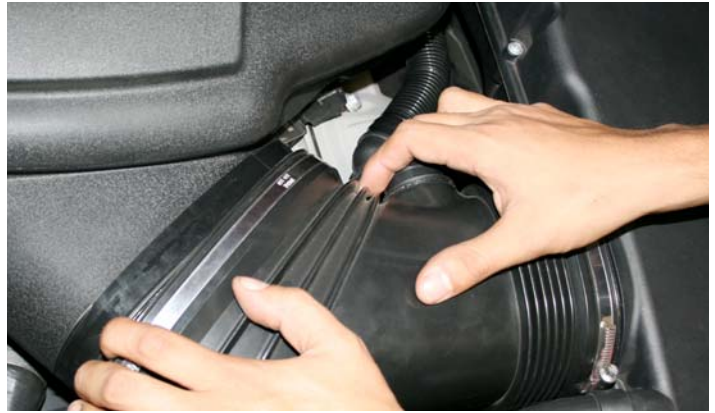
5- Gently pull the intake tube off of the intake plenum.
