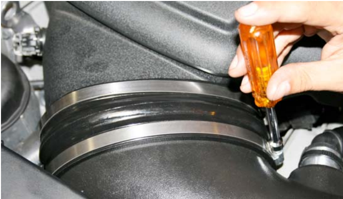
25- Tighten down both clamps on supplied coupler using a 5/16" nut driver to secure intake tube to intake manifold. Note: Do not over tighten.
