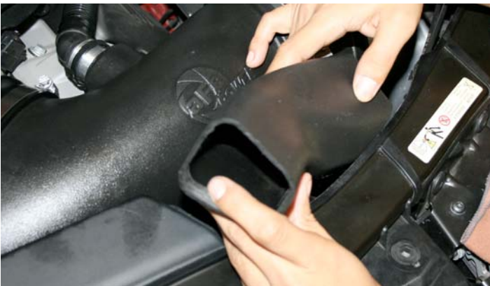
20- Place the cold air duct into the housing slot, and work it into position.
