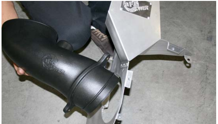
8- install aFe's intake tube into the housing.
