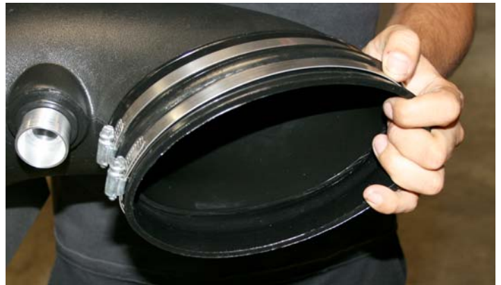
13- Position coupling onto intake tube with supplied clamps. Do not fully tighten.
