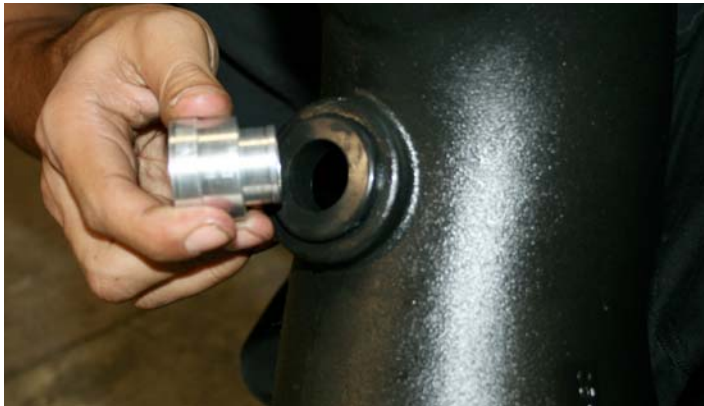
11- Firmly press the adapter into the grommet until it is seated all the way in.
