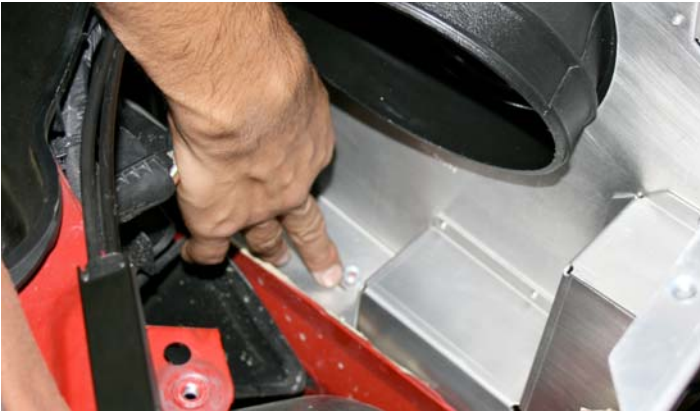
17- Place the supplied nut with wavy washer onto the bottom of the housing. Do not fully tighten.
