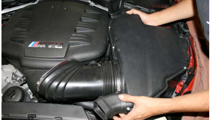
6- Pull up on the back of the intake and work the intake free from the engine bay.
