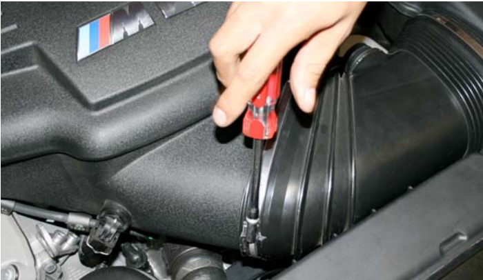
3- Loosen the intake tube clamp from the intake tube with a 1/4" or 8mm nut driver or flat head screw driver.
