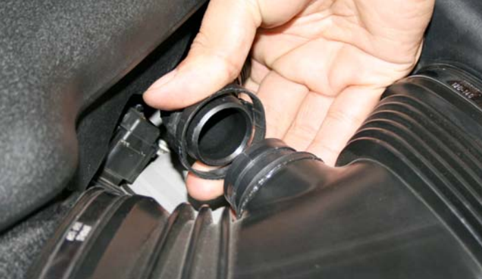
2- Gently squeeze the stock smog pump and pull straight back to remove.
