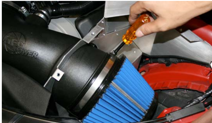
27- Once filter is in position, tighten clamp with a 5/16" nut driver. The white filter is oil-free and is included as a spare filter. The white filter is washable but should not be oiled.
