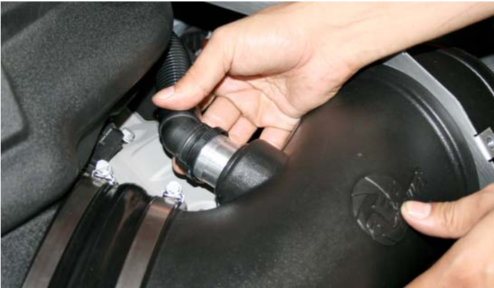
19- Insert the smog pump line onto the adapter and make sure it locks into place.
