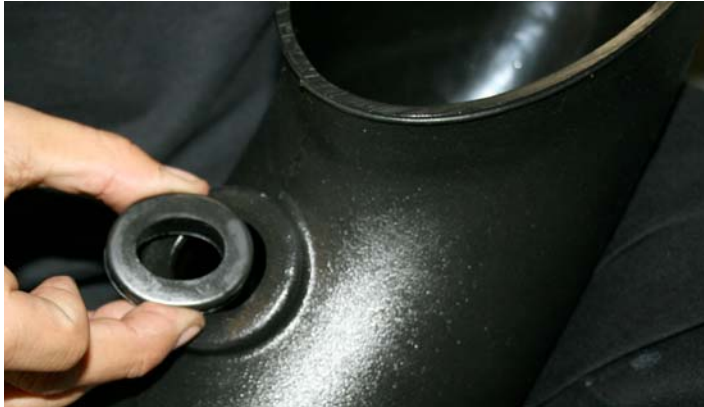
10- Install supplied grommet into aFe's intake tube.
