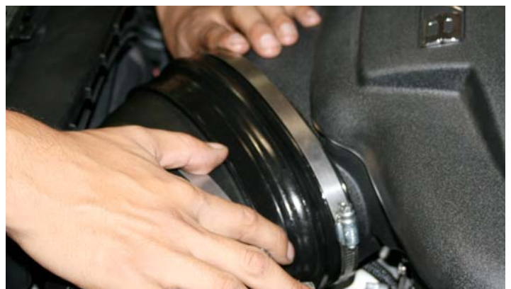
16- Slide the coupling onto the intake plenum, use the bead on the tube to verify that the coupling is on straight. Do not fully tighten.
