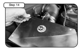
Install cover using button head screws provided and tighten using 5/32" allen key. Re-connect MAF sensor
