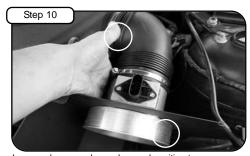
Loosen clamp on plenum box and position to new adaptor. Do not tighten.
