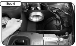
Install housing into vehicle.
