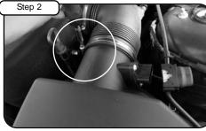
Disconnect MAF sensor harness. Loosen clamps with 1/4" nut driver. Pull back vacuum line.
