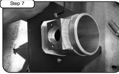
Install filter adaptor to housing using 4 button head screws & wavy washers. Tighten using 5mm allen key.
