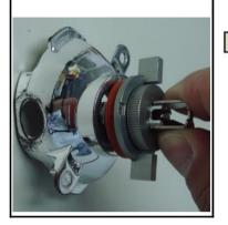
into the positioning slot of Lamp Cup
