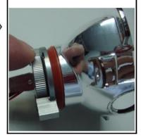
g). Turn and adjust LED Bule to the light source position and fix ( Front view)
