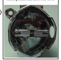
h). Turn and adjust LED Bule to the light source position and fix it (side view)
