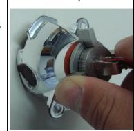
e). Rotate LED Bule to position but LED light source position is not at proper position.
