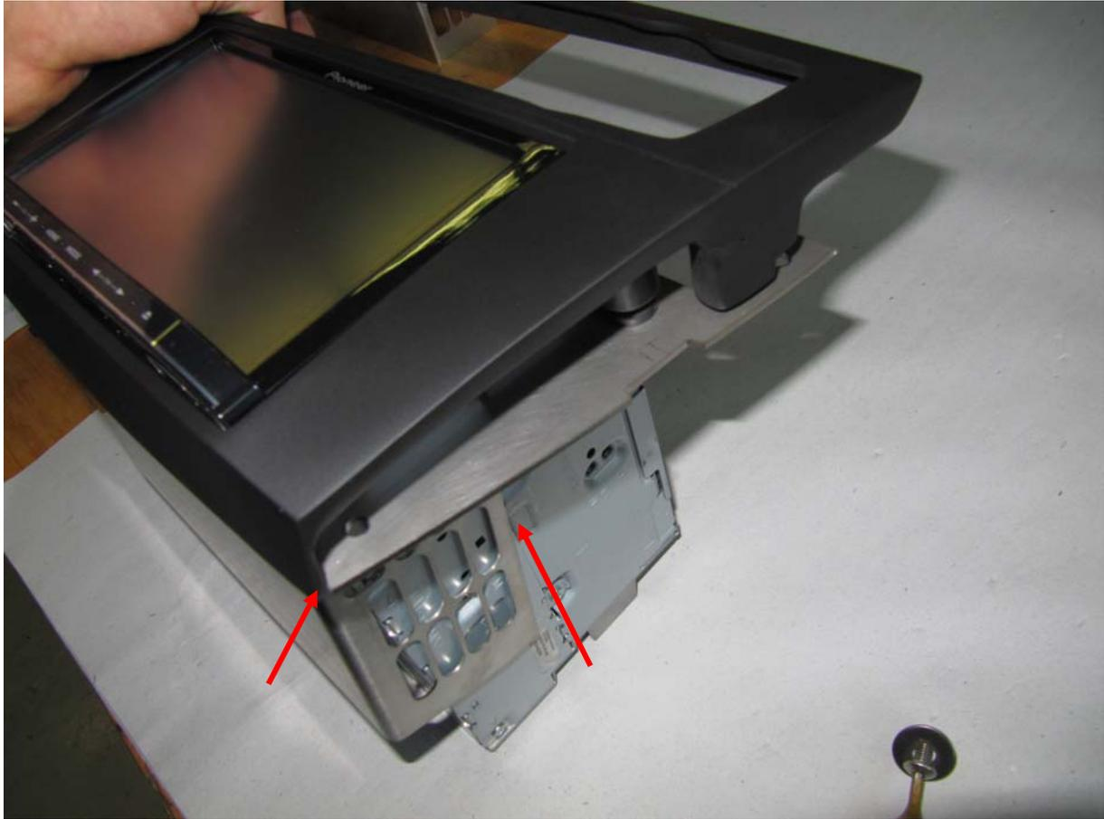
4: put I the double-din device now from the backside, look after that the bottom border is still same as metal border
