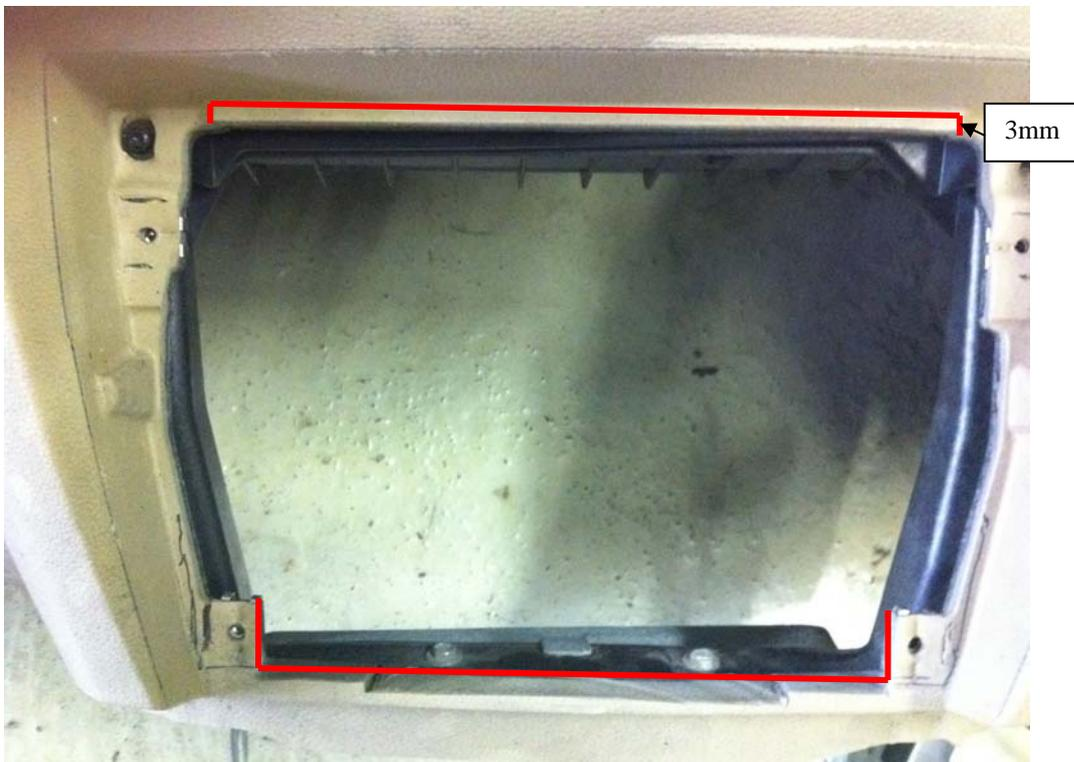
13. cut out the dashboard like red line with a dremelike tool, at top only 3mm high for ac-control
