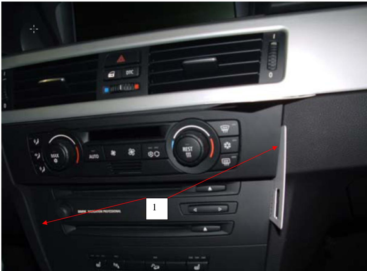
1: demount the front panel with a check-card, its just pined
