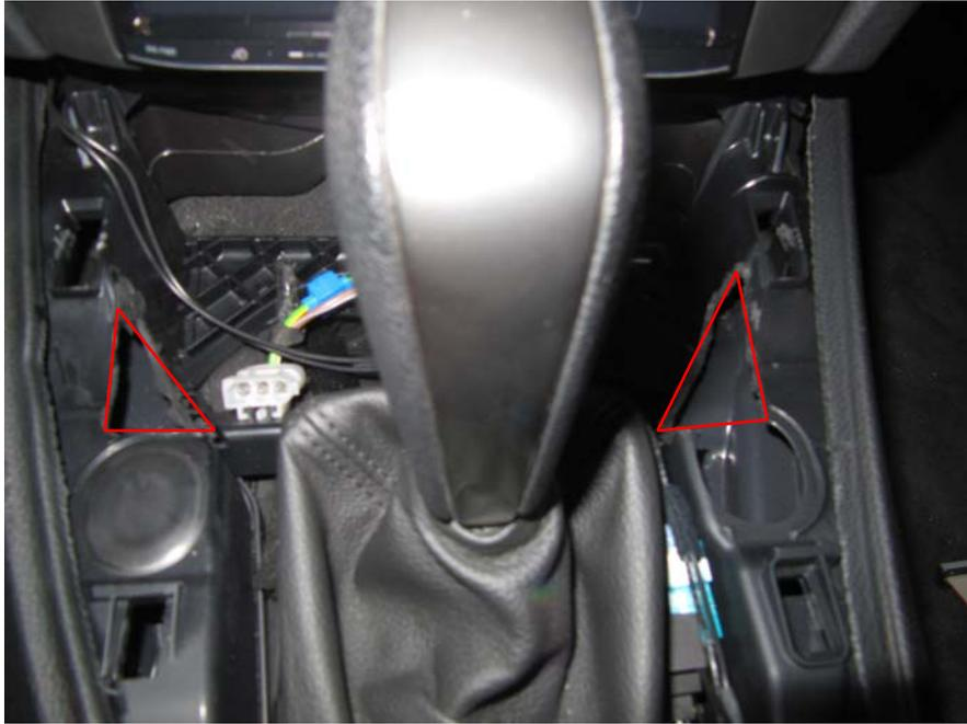
12. cut out the middle tunnel for the multi-button bar like red line, depth 20mm
