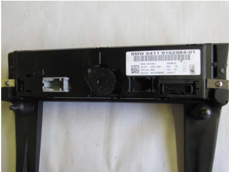
2: Demount the ac panel and screw it backside at the bezel, use the small inox plates, turn the longer sides of the plates to the center and screw them down with 2,9 x 13 mm screws.
