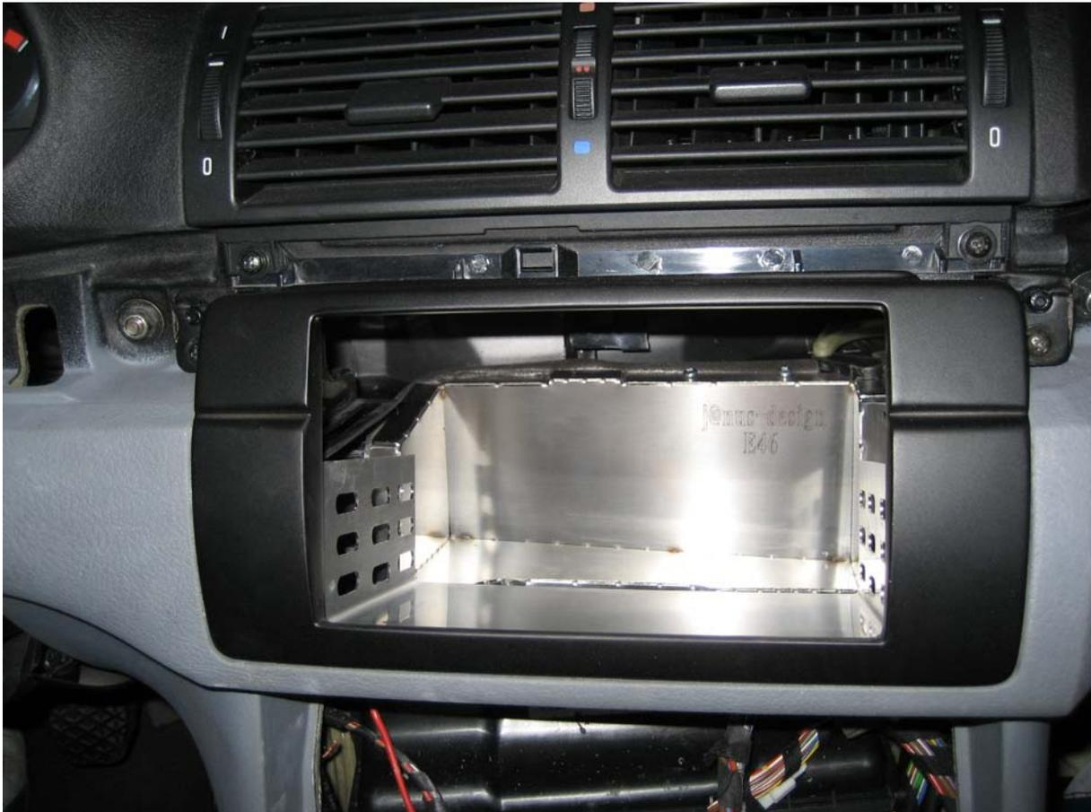
Softly press the D-DIN bezel inside the dashboard that and fix it with the screws. Don't screw them to endpoint, just that they are flush
