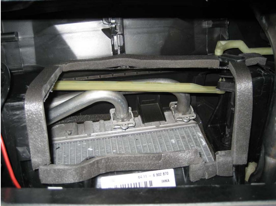
glue the sealing foil at the revolving border
