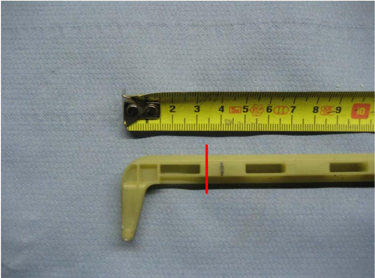
Cut the vent-arm at the left side 3,5cm at the left end with a dremel or saw, drill 2mm holes central at both sides
