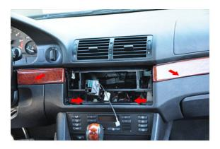
1. Remove the original radio, and take the screws out as marked in picture
