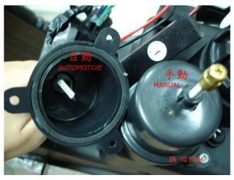
4. Please find the wire from the original one and connect with the white connector that on the picture. After you connect the connector, everything is OK and Finish  $\sim\sim$
