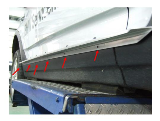
4. Both front and back sides need to be locked. There will be 22~24 screws enclosed, and then the installation is done.
